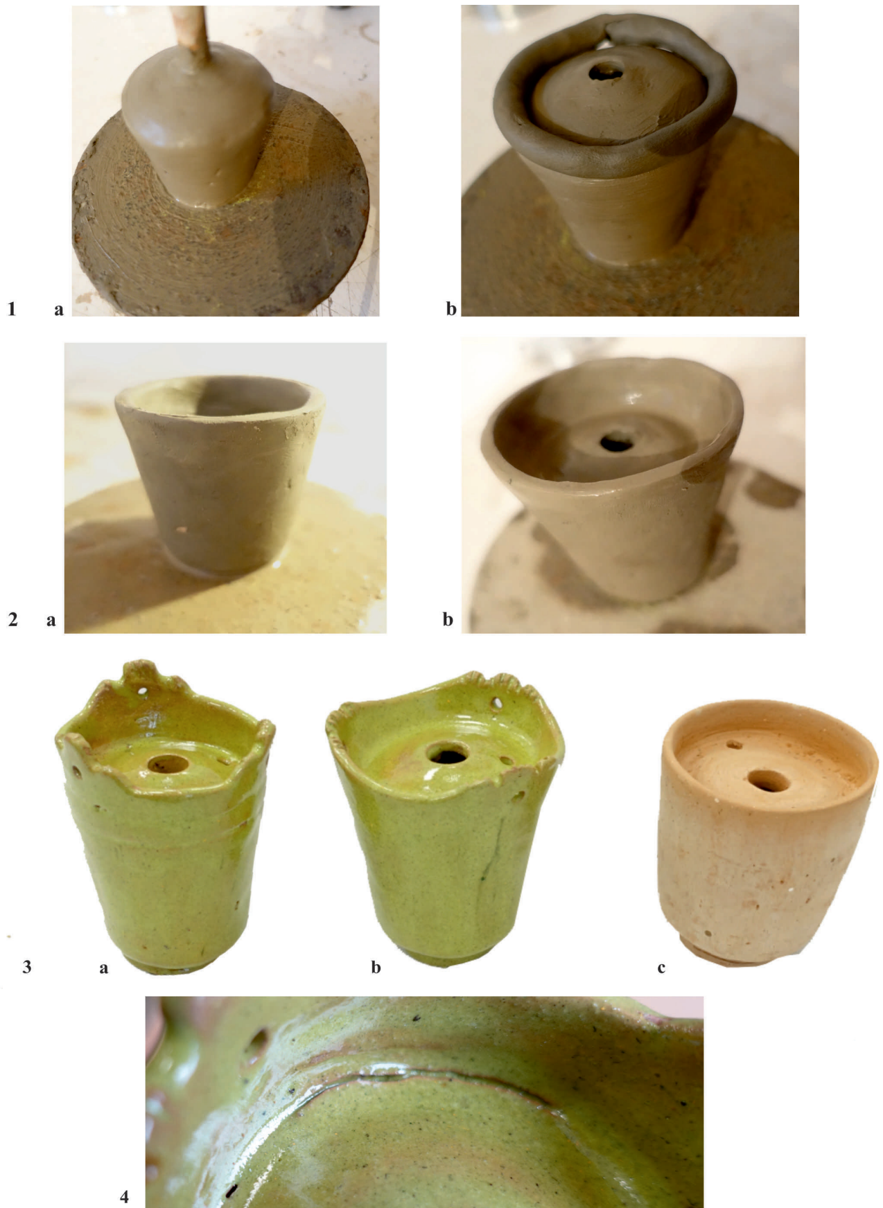
Fig. 10. Experiments to model some inkwells. 1a-1b Direct modelling of the lid. 2a-2b. Application of the lip that was manufactured separately. 3a-3c. Inkwells after glazing (3a-3B) and firing. 4. Crack appeared on a piece modelled using variant 2.
