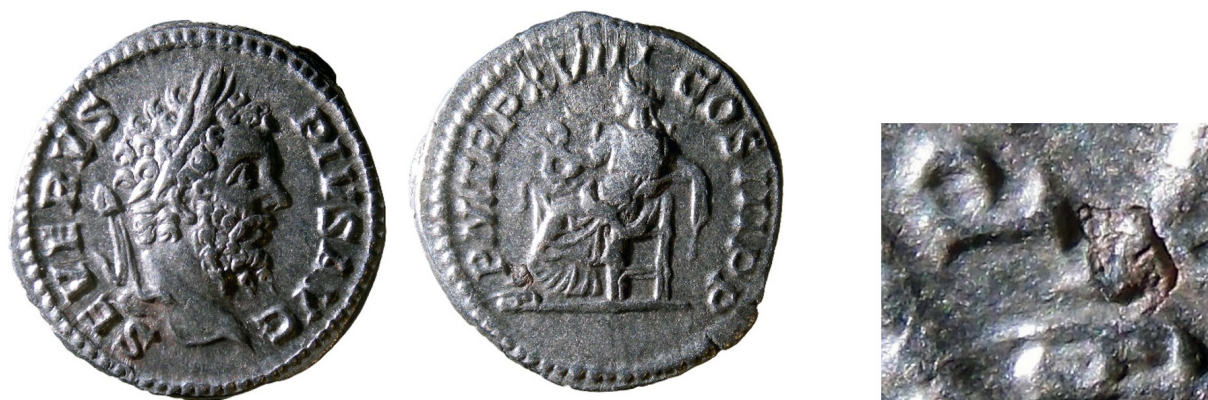
Fig. 1. Denarius Septimius Severus. The minuscule spot with the missing silver foil reveals the copper core.
