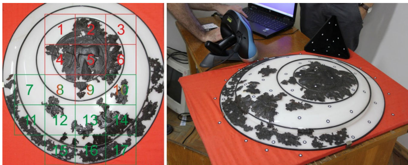
Fig. 4. Laser scanning of the fragmented disc using ViusCAN.
