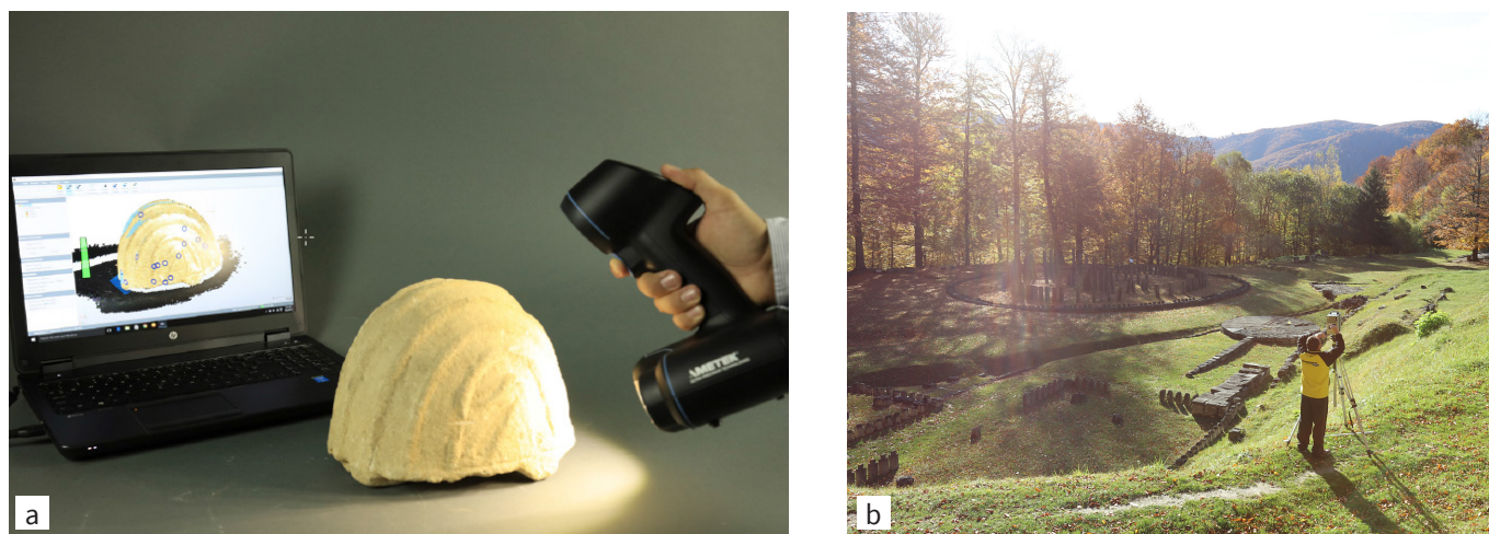
Fig. 6. Aspects during the digitization process: (a) The 3D scanning of a limestone hemisphere using a structured light scanner; (b) The 3D scanning of the Sarmizegetusa Regia Sacred area, using a terrestrial laser scanner.
