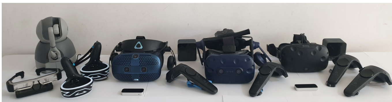
Fig. 9. Some of the hardware equipment used for the digital applications, starting with tracking sensors, haptic devices, and various head mounted displays suited for virtual reality applications.
