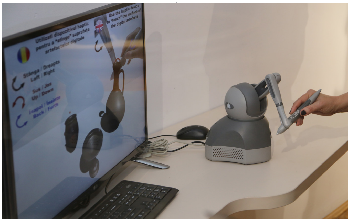
Figure 1. The proposed equipment and application that enables tactile experiences with digital artefacts.
