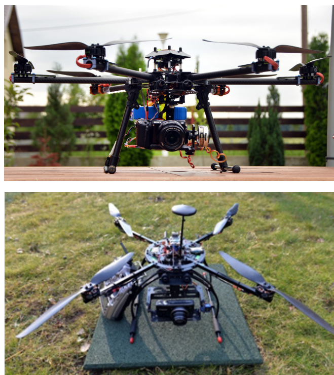
Fig. 4. UAV platforms developed in the project: up - H1D1; down - Q1D2
