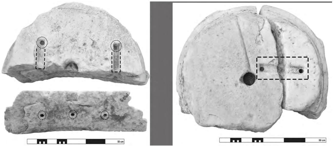
Fig. 8. Repairs detected on attic-ion type pedestals belonging to the emperor's hall of the gymnasimun in Side (after YURTSEVER 2021a, Pl. 11,3; 27,2).
